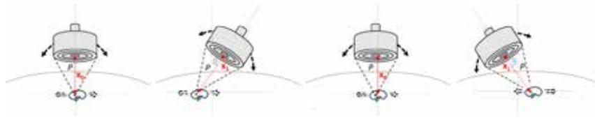
Figure 2. Schematic representation of the angular motion compensation strategy used for FUS therapy of moving targets. The transducer rotates around a pivot point (P) chosen at will, and focal depth is continuously adjusted utilizing the electronic steering.
