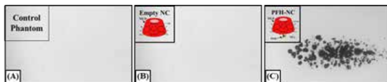
Figure 2. 15MPa pulses applied to tissue phantoms containing (A) no particles, (B) empty NCs, and (C) PFH-NCs.
