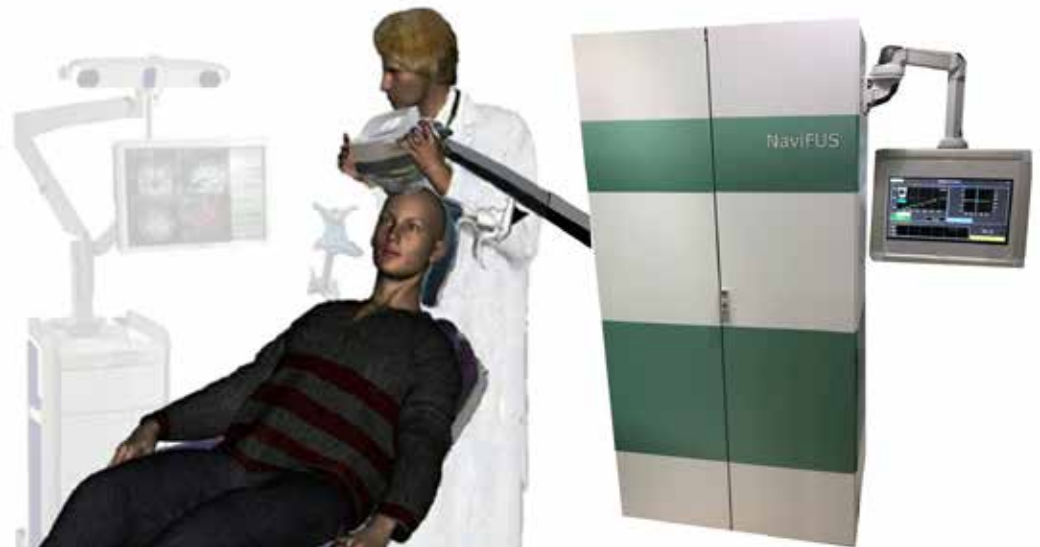
Figure 1. NaviFUS: A Neuronavigation-Guided Focused Ultrasound Device for Clinical Transcranial Brain Application
